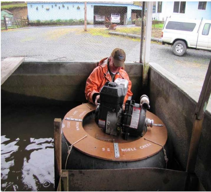
Greg Brown installs pump on a float getting ready to vacuum mud and waste off of the bottom of Nora's Pond.
