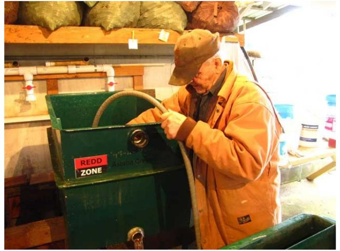
Clyde hoses out mud from the top using a spray nozzle. We also insert the spray nozzle through the two inch pipe at the bottom of the hatch box. That gets most of the mud out.
