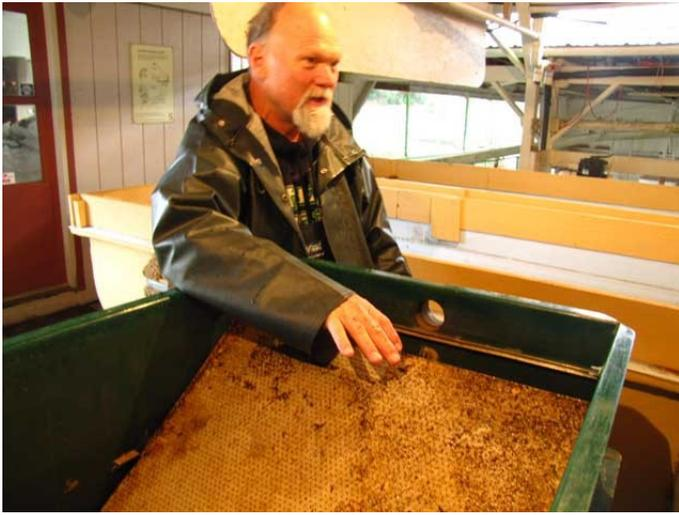
March 9th was a work party day to clean out all of the hatch boxes. There is a lower screen that the bio rings sit on. The mud settles on the bottom under the screen. We removed the screws from one tank and took the screen out. We decided it wasn't worth the effort required to remove the screen.
