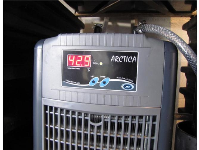
This is the chiller from Tod Jones at Redd Zone. The water temperature in Noble Creek is 42.9 degrees. We need the chiller to bring down the temperature by five degrees and hold it for twenty four hours to mark the otolith of the Coho being hatched. The chiller at 10:45 AM was 42.9 and at 5:00 PM it was 36.5 degrees when Clyde turned it off. It took longer than we anticipated to get the five degree drop but we got there!
