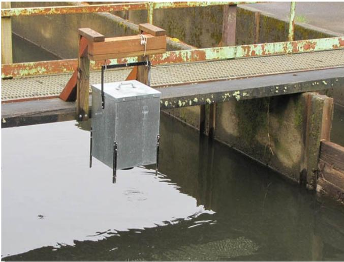
The automated feeders have finally been installed. The very smallest feed won't feed correctly in the feeders. Clyde has to feed by hand for the first few sizes of feed before these feeders will work correctly.
