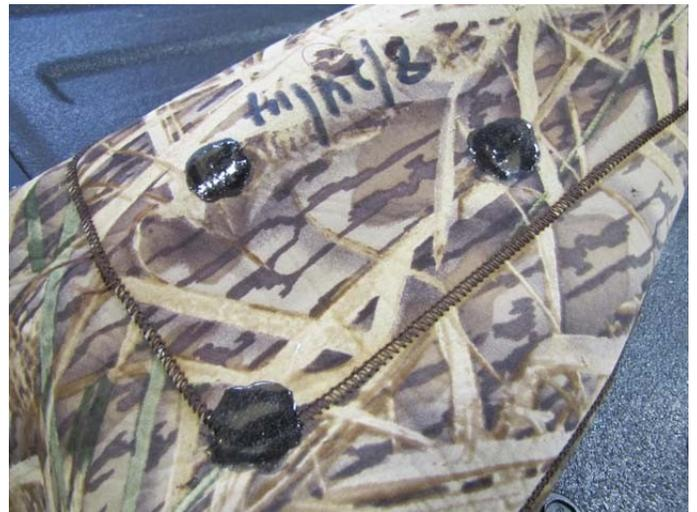
This set of waders has been repaired using Aquaseal from BiMart. The Aquaseal is applied as a blob about 1/4" larger than the hole. It then spreads and penetrates the neoprene before drying to a hard flexible patch. All five sets of waders were repaired successfully.
